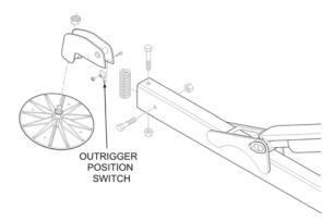
Figure 4-1. Outrigger Position Switches
